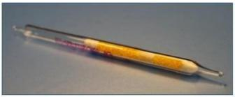
Description: Glass tube containing a granular absorbent and glass wool filter. Active pump sampling using preset air pumps.
