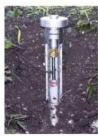
7. Push the assembled Soil Probe cap unit into the Soil Probe. The unit is now ready for sampling (sampling period of 1-4 weeks). Mark or record the location of the Soil Probe for easy identification at the end of sampling.
