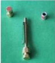
1. Identify the end of the tube with the groove (usually the end with the colored spot on the cap).
