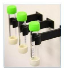
**Description:** Acrylic tube fitted with green and white thermoplastic rubber caps. The colored cap contains the absorbent. A one-micron porosity filter is fitted to prevent particulate ingression.
